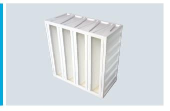
Introduction of Fine HVP is to replace the conventional box style Medium Filters ranging from M5 to F9 grades. Fine HVP operates at very high approach velocity of 3.75 m/s if required delivering a very low pressure drop. The V shaped arrangement allows more air flow per filter wherein a standard filter replacement can save energy up to 30%. Filters are light weight and its fully plastic body makes it incinerable as well.
